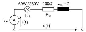
Calculate the nessesary value of the inductivity L of the coil, for operation the filament lamp with its nominal values!
