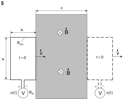
The wire-loop (a = 50mm, b = 30mm) is moved with a speed of v = 0,2m/s through the homogeneous magnetic field (B = 1T, c = 60mm).
