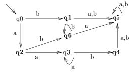
Figure 13: Deterministic finite state automata (accepts  $a^*b + ab^*$ )
