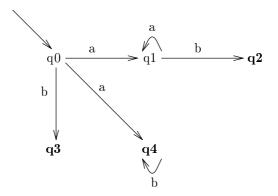
Figure 14: Nondeterministic finite state automata (accepts  $a^*b + ab^*$ )
