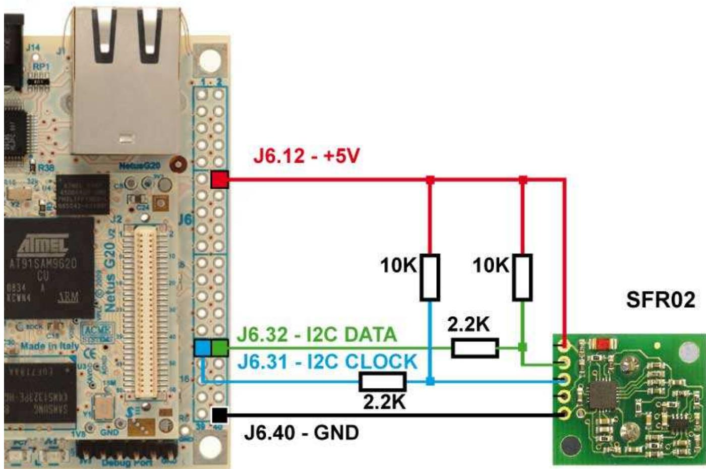
Be carefull to insert the 2K2 resistors to avoid damage on the FOXG20 GPIO lines that are at 3.3 volt
