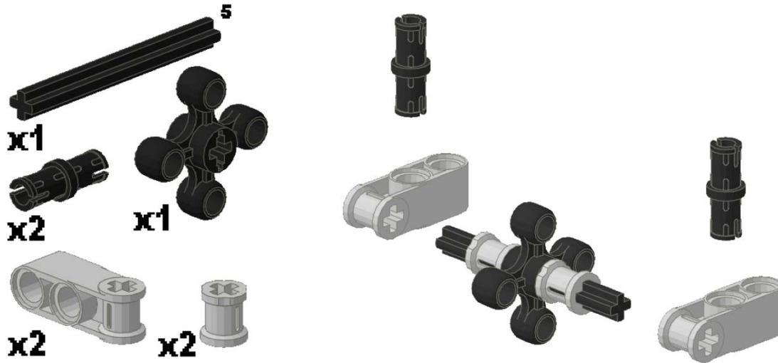
Slide a 5 stud axle through the skid. Side on 2 half bushings to keep the skid centered followed by 2 axle joiners on each end. Place a friction pin into the middle hole of the axle joiners.
