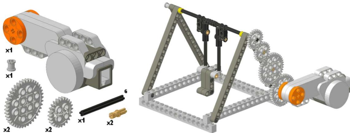
Place 1 of the 24-tooth gears on the exposed 10-stud axle at the top of the assembly. Connect the other 24-tooth gear using the axle pin to the 4<sup>th</sup> hole from the top of the beam. Connect one of the 40-tooth gears to the 8<sup>th</sup> hole from the bottom of the beam. Connect the other 40-tooth gear to the 2<sup>nd</sup> hole from the bottom of the beam using the 6-stud axle to the motor. Secure the motor in place with a bushing.
