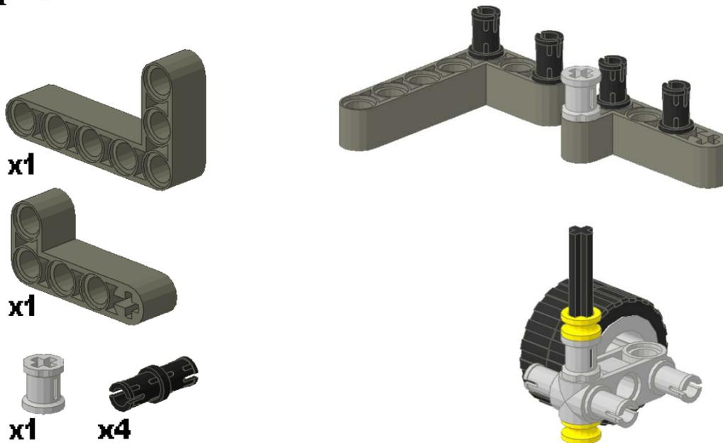
Take a small L-beam and attach 2 black friction pins to the 2nd hole and the 2nd hole from the top. Attach that to the parts from Step# 1 with a bushing. Take an L-beam and attach 2 black friction pins to the 2nd and 3rd holes.
