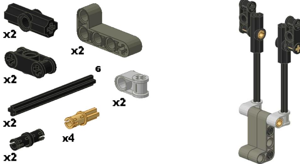
Connect the 2 lift arms using 2 axle pins. Place an axle pin with friction into the top holes of the lift arms. Connect these pins to the gray axle joiners. Insert a 6 stud axle into each axle joiner. Place a gray connector on each axle. Connect the black axle joiners using the 2 stud axles.
