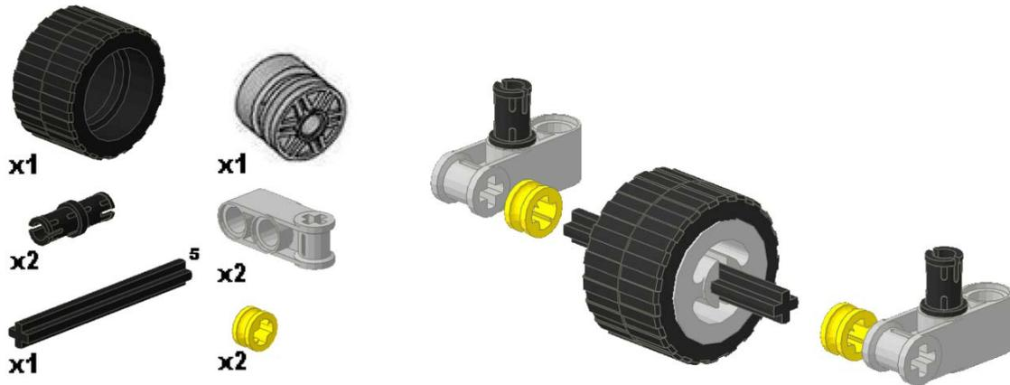
Slide a 5 stud axle through the wheel. Side on two half bushings to keep the wheel centered followed by two axle joiners on each end. Place a friction pin into the middle hole of the axle joiners.
