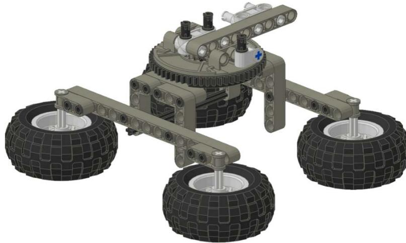
Use the assemblies from Steps #1 and #2 to assemble the complete base. For added support, take a 12-beam and connect it between the 2 sides of the base.
