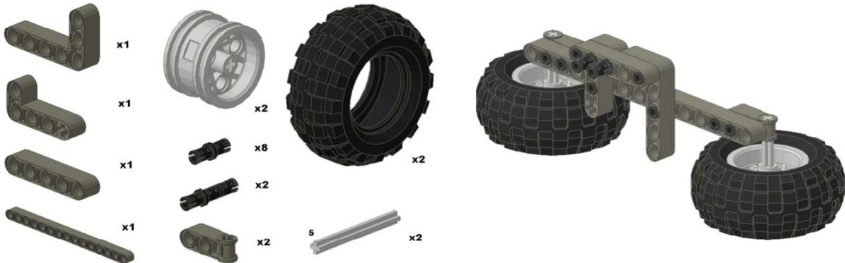
Construct supports for the base of the merry-go-round. Use wheels for the bottom, axles as attachments, an assembly of beams and pegs as the supports. You will need 2 of these assemblies to create a sturdy base.
