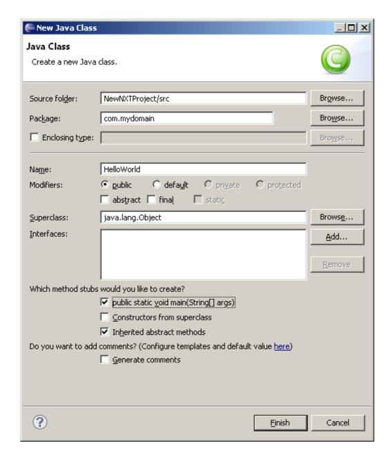
Enter a package name and the a the name of the class. In the example, the class name HelloWorld has been chosen. The package name com.mydomain corresponds to the DNS domain "mydomain.com".
