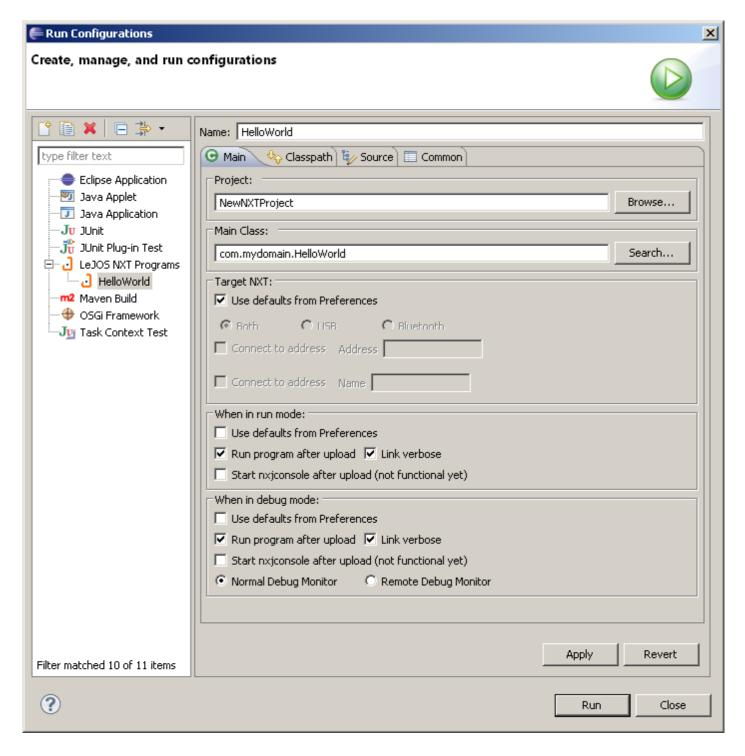
After making the changes, click "Apply" and then "Run" or "Close". After enabling the verbose linking, the output in the console window when uploading a program to the NXT will change:
