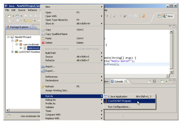
You will see output on a leJOS NXJ Console. Also note, that two additional files have been created in the project root directory. The nxj file is the one being upload to the NXT brick. The nxd is for debugging purposes.
